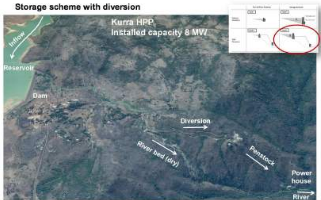
Figure 57: Hydropower plant type “Storage scheme with diversion”. Example Kurra HPP in Nigeria.
