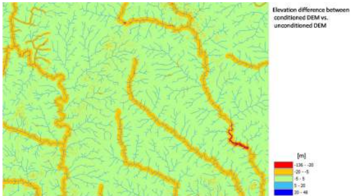
Figure 27: Comparison of elevation data from Hydrosheds conditioned and unconditioned 3s DEMs. Example for region in Burkina Faso. Yellow areas indicate stream burning by 5 to 20 m. Red area shows extensive stream burning (more than 20 m) at an existing reservoir (Bagre reservoir).
