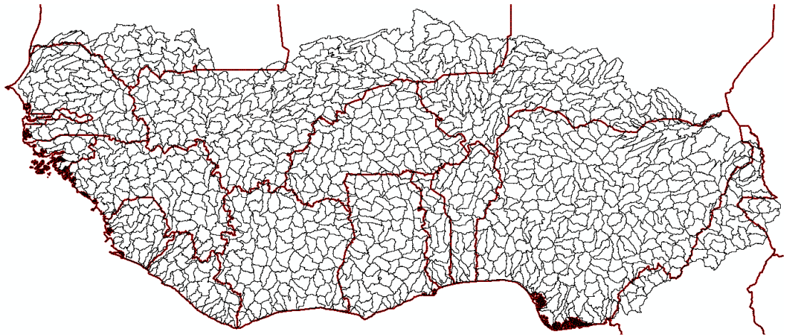
Figure 66: Layer D3 sub-areas consisting of 1060 sub-catchments. Red: country borders. Black: sub-catchment borders.
