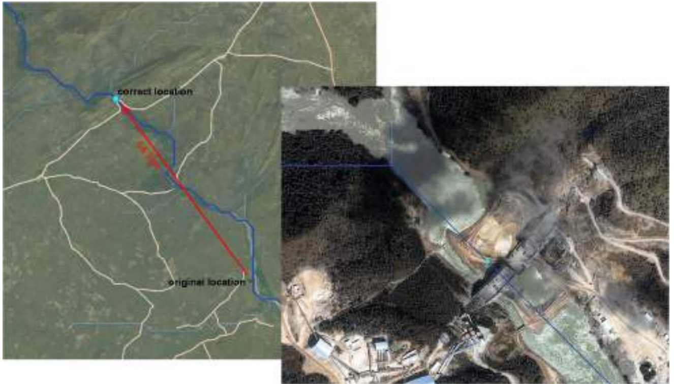
Figure 1: Manual geo-referencing of existing hydropower plants by use of satellite images. Example for the recently constructed Bui HPP in Ghana. Here, the HPP was misplaced by 14 km with the originally reported coordinates.
