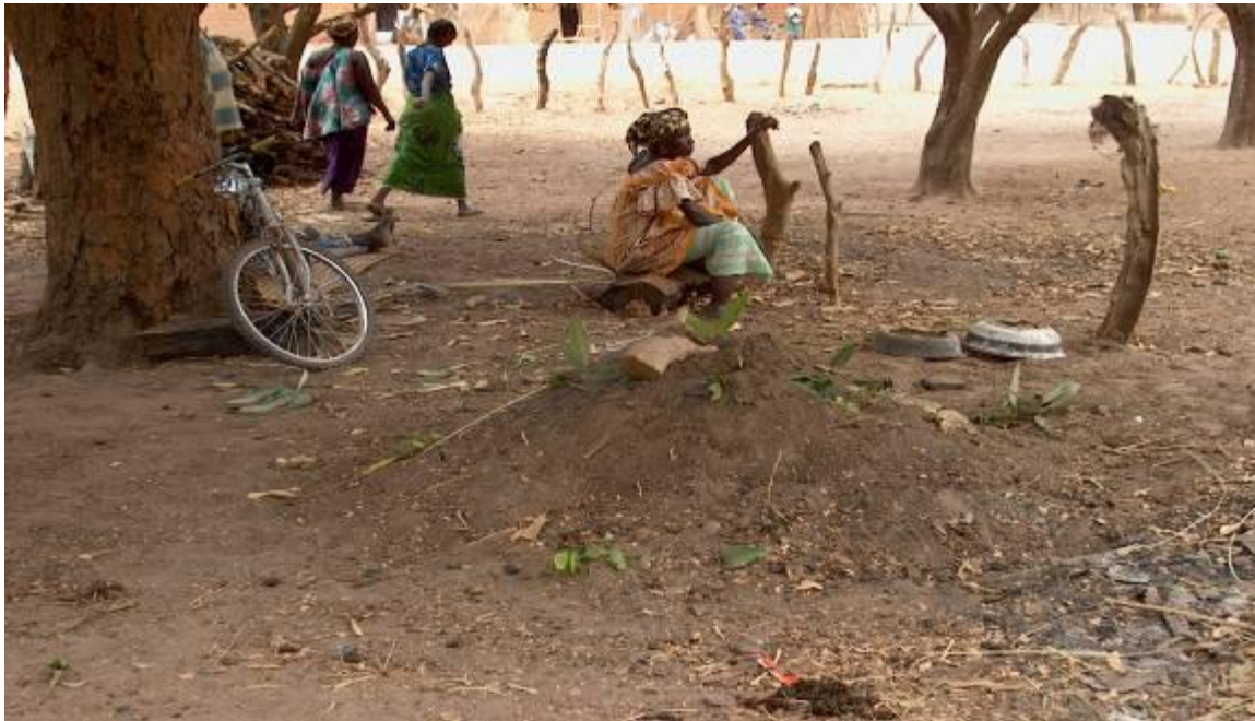
Figure 6.1: Traditional Earth Kiln for Subsistence Charcoal Production
