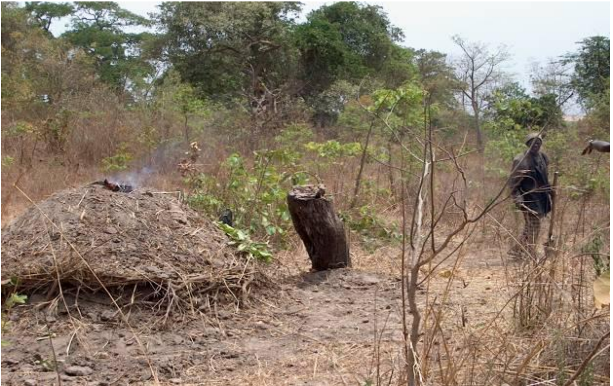
Figure 6.2: Traditional Earth Kiln for Commercial Charcoal Production
